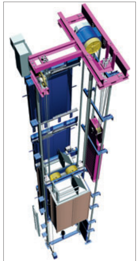
Fig. 4: The highly flexible LiftEquip MRL set made to order
